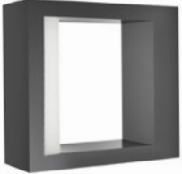
[ BLISS 819502 ] Dark Gray Aluminium Acrylic Diffuser LED 7 Watt 560Lm CRI>80 220-240 Volt 50Hz Beam 56° IP54 3000K or 4000K AC Driver Included L: 15 W: 6 H: 16 cm
