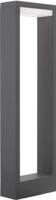
[ BLISS 819503 ] Dark Gray Aluminium Acrylic Diffuser LED 7 Watt 560Lm CRI>80 220-240 Volt 50Hz Beam 56° IP54 3000K or 4000K AC Driver Included L: 15 W: 6 H: 50 cm
